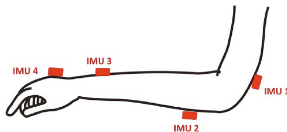
Figure 20. Location of inertial sensors to calculate wrist and elbow rotations by differential measurement.
